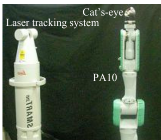
Fig. 1. Experimental setup for measuring position of robot arm's tip
