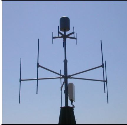
Fig. 6. Five element Uniform Circular Array interferometer
