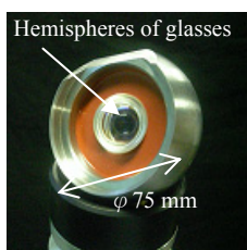
Fig. 1. Experimental setup for measuring position of robot arm's tip
